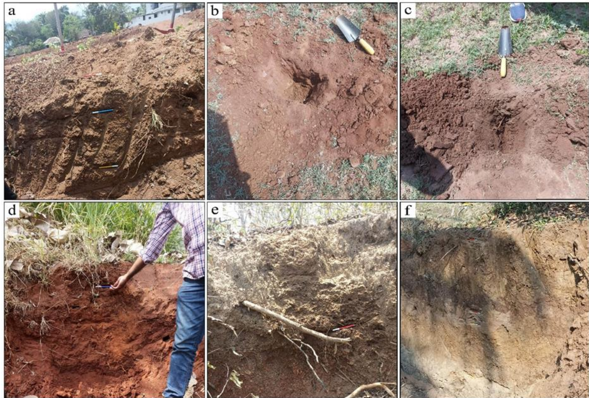
Figure 3. a) shows the soil collected from Kollenkode, Kerala area. b) The soil from the Pollachi, Tamil Nadu area shows a fine texture with few granules. Topsoil is removed by a steel scoop and the fresh portion of the soil is collected from this small pit c) The top portions of the soil are removed from the steel scoop and the fresh portion of soil is collected from Avalchinampalayam, Tamil Nadu area. The soil shows moisture content and is slightly reddish-black in color due to the oxidation and organic content of the soil. d) The photograph shows reddish lateritic cover soil collected in a field from Santhegoundampalayam, Tamil Nadu. e) The photograph shows the fine and coarse texture of soil at the top and the bottom of the soil profile, respectively. The top portion is slightly leached, and the bottom coarse grains show oxidized coatings in this soil profile where the soil collected from Vadakarapathy, Kerala. f) The photograph shows fine texture and moderately compacted soil due to the mixed portions of clay in the soil profile. The soil profile shows dark thick clay interbed (red pen indicates the bottom of clay bed) within the topsoil and bottom leached soil. The soil is collected from Kollengode, Kerala.
